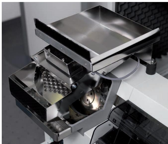
by denomination by the PREMA machine. Staff at the bank counter can empty the machine as and when required by opening its lockable front doors.
